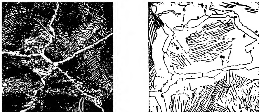
FIGURE 493. Metallographic structures of typical examples of (left) normal and (right) abnormal steels after standard McQuaid-Ehn treatment. Etched with picral. \times 1000 , originally; reduced about one half in reproduction. (Photomicrographs courtesy U. S. Steel Corporation Research Laboratory, Kearny, N. J.)
